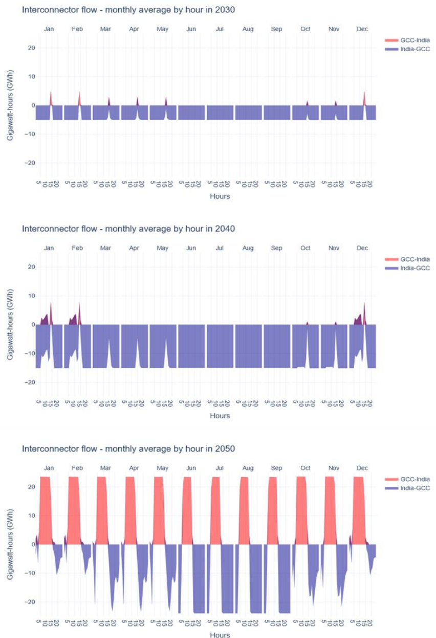
Figure 2: Hourly bi-directional trade volumes across the GCC-India interconnector in 2030, 2040, and 2050 (Primary x-axis: Hours [0-24]; Secondary x-axis: Months; Y-axis: Gigawatt-Hours [GWh])
